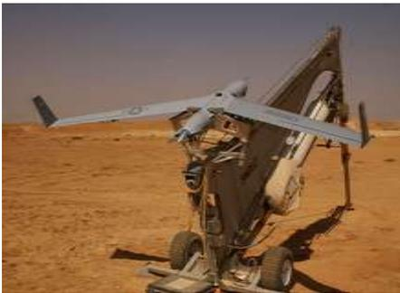
Boeing's Tactical Compact Communications Relay (TCCR) allows a small UAV to function as a communications repeater for military handheld radios. It can extend the range of line-of-sight (LOS) handheld tactical radios to more than 150 nautical miles and is small enough to fit into a slot of about 5 by 5 by 1 inch in the **ScanEagle's** payload bay.
