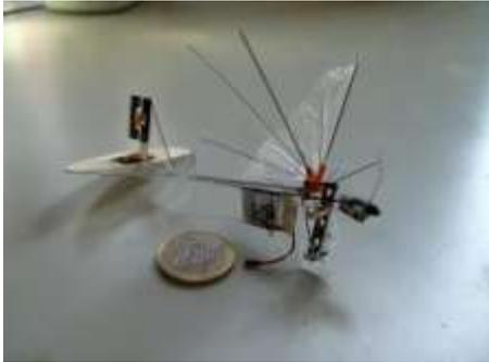
The **DelFly Micro** is a 'Micro Air Vehicle' (MAV), an exceptionally small remote-controlled aircraft with camera and image recognition software. The Micro, weighing just 3 grams and measuring 10 cm (wingtip to wingtip) is the considerably smaller successor to the successful DelFly I (2005) and DelFly II (2006). (Credit: Image courtesy of TU Delft)
